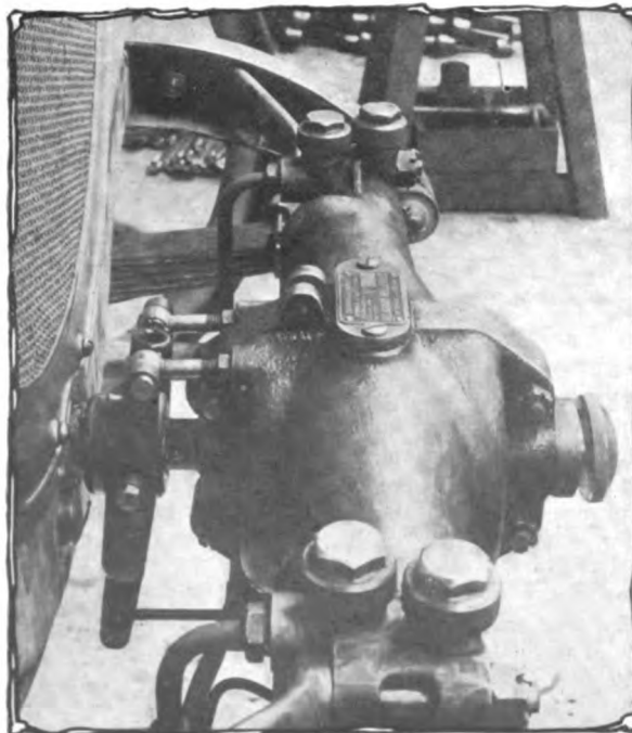
Compressed air starter on the Delaunay-Belleville
